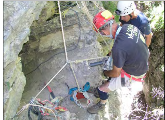
At Fantoms Hole entrance, reception of the UGPS signal sent by the transmitter located underground [photo. J.-Y. Bigot]
